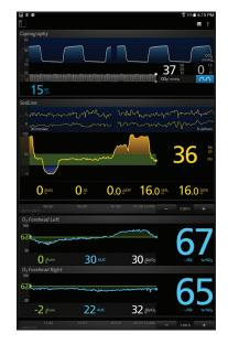
Display data from modules connected through MOC-9<sup>™</sup> ports to Root<sup>®</sup>, such as SedLine<sup>®</sup> brain function monitoring, O3<sup>™</sup> regional oximetry, or an ISA<sup>™</sup> EtCO2 module
